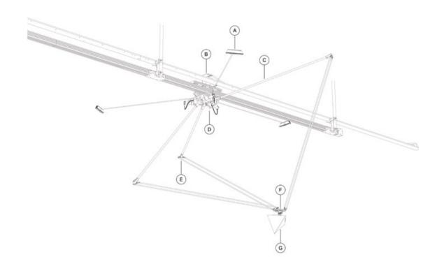
Annotated illustration of the 5-metre (16-foot) tall custom-built delta robot: (a) Kinect sensor array; (b) 21-metre (69-foot) linear carriage; (c) carbon-fibre structure; (d) central robotics platform; (e) parallel mechanism; (f) pan and tilt servomotors; (g) electroluminescent tetrahedron.
